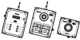
Upon activation of the First Aid manual Call Point, the audible sounder will sound (buzzer tone) and the **i** Status LED will flash. Upon activation of the Fire manual Call Point, the audible siren will sound (sweep tone) and the beacon will flash. Note that, in the case of activation of both First Aid and Fire manual Call Points, Fire takes priority.
